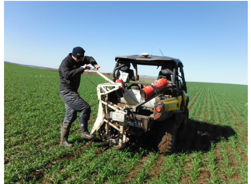
ABA State-wide acid soil project, Precision Agriculture using soil-pH machine
